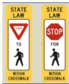
In-Street Pedestrian Crossing Signs
